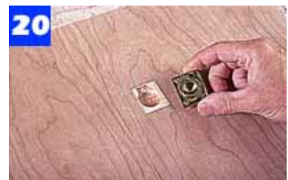
Cut a mortise in the drawer face for the ring pull. A 1-in.-dia. recess in the center of the mortise fits the body of the pull.
