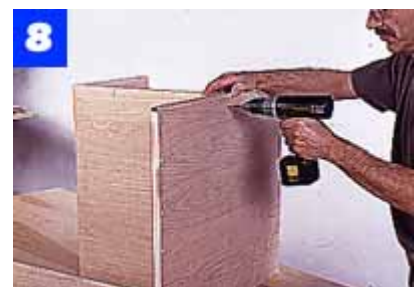
Use plates and glue to build the L-shaped section of the drawer box. Use dry plates and screws to attach to inner case side.
