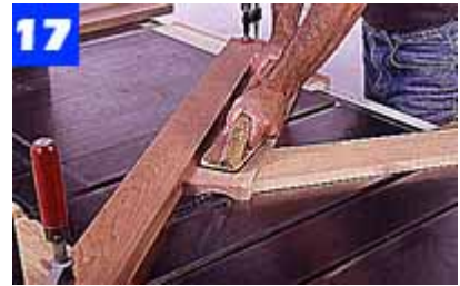
Use a wooden fence angled across the saw table to guide the stock for a cove cut. Increase blade height in 1/16-in. increments.
