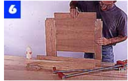
Apply glue to mortises and tenons and join rails to one stile. Slide panel in place, add remaining stile and clamp until glue sets.
