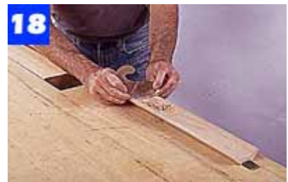
Use a gooseneck scraper to remove saw marks from the face of the cove molding. Then, sand with 220-grit sandpaper.
