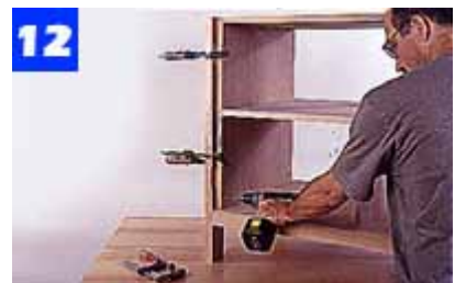
Slide the inner case into position between the lower case outside frames, and clamp. Screw the inner sides to the outer frames.
